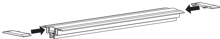
5. Slide the spring toggle mounting brackets onto the profiled bar, aligning
