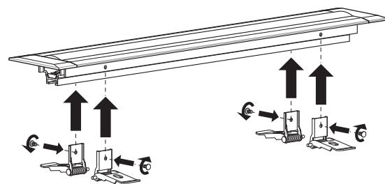
6. Tilt in the bracket arms and pass the lighting fixture through the hole in
